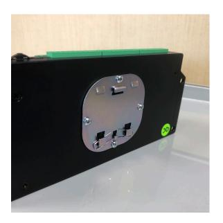
9) Attach the eGauge using the included DIN mounting kit. The mounting kit can be used to orient the eGauge in many ways. The image to the left shows a "flat" mount.
