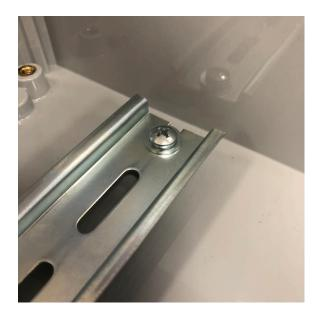
2) The two 13" pieces of DIN rail should already be mounted in the enclosure. With a Phillips head screwdriver, check to make sure they are tightly screwed in place.
